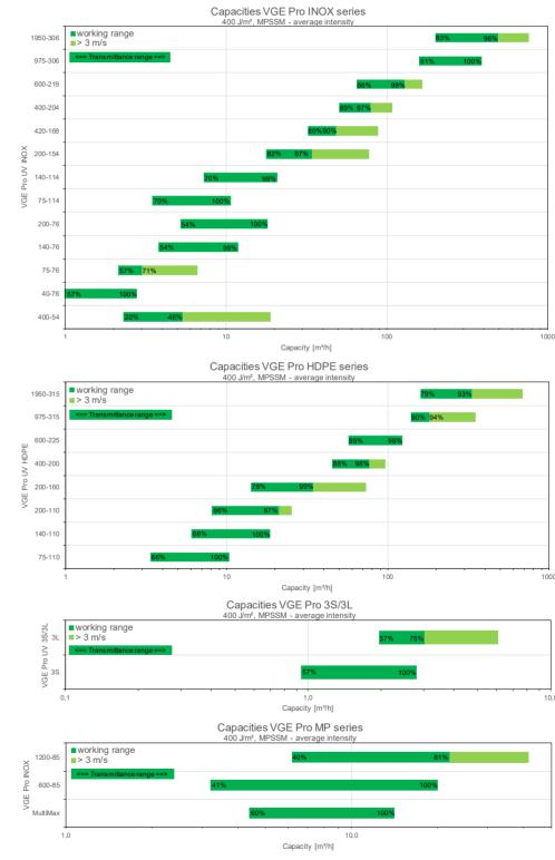
$An \, UV-C \, dose \, of \, 400 \, J/m^2 \, equals \, 40 \, mJ/cm^2 \, and \, the \, transmittance \, of \, the \, water \, is \, measured \, with \, UV-C \, light \, (254 \, nm) \, through \, 10 \, mm \, of \, water.$
